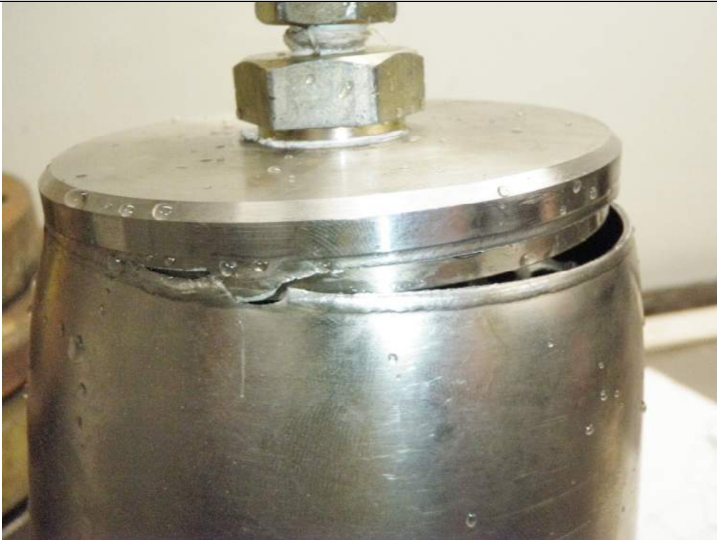
Photo 3 – After test, Failure along weld of end cap
