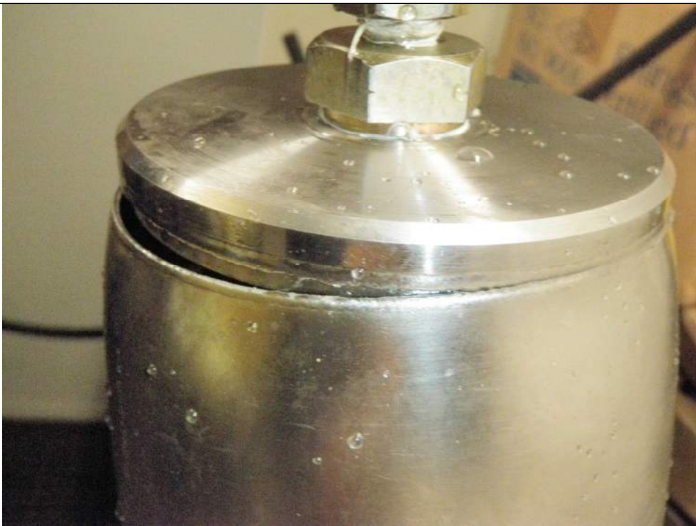
Photo 4 – After test, Failure along weld of end cap
